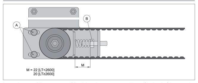
Loosen the screws [A], unscrew screw [B] until the spring compresses to 22 mm (if the length of the automation is less than 2600 mm) or 20 mm (if the length of the automation is more than 2600 mm). Lock the adjustment by tightening screws [A].
