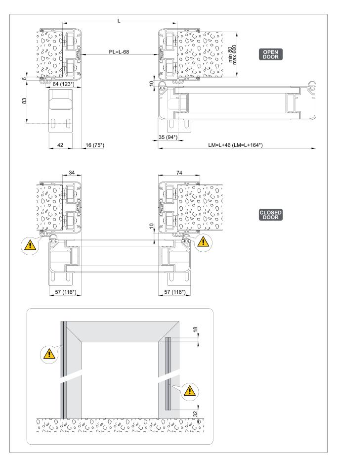
NOTE: the figure refers to doors that open to the right. For doors that open to the left, the position of the door stop profiles must be reversed.
