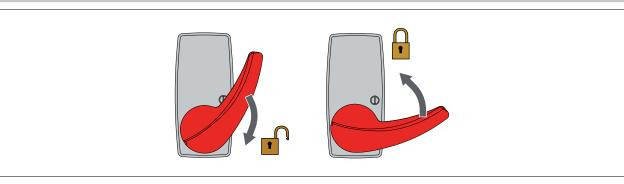
In the event of maintenance, malfunctioning or emergency, pull the lock release lever LOKSBM down (if installed) and move the door wings manually into the open position.
