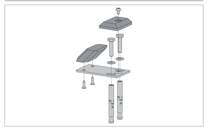
Install the floor guide for the PAMH60 door wing by complying with the measurements on page 8 [VALORHH], or on page 10 [VALORHS].
