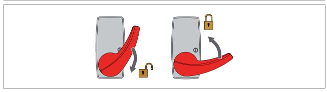
In the event of maintenance, malfunctioning or emergency, pull the lock release lever LOKSBM down (if installed) and move the door wings manually into the open position.
